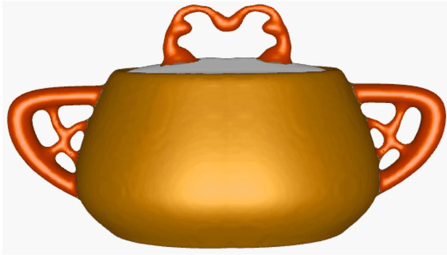
Figure 4.34: The teapot model is modified to create a decorative two-handle teapot. The spout and top handle are erased and new handles are added. Edits are made to one side of the model and a volumetric reflection operator is used to create the symmetric result.
